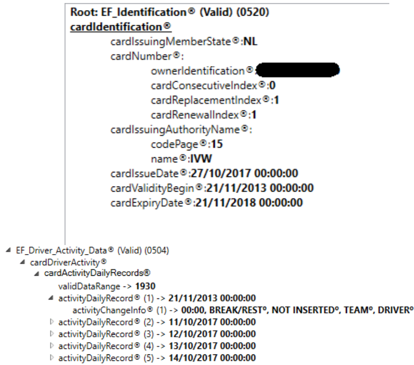
Figure 4.7: EF_Identification and EF_Driver_Activity_Data data from a driver card issued in the Netherlands.
